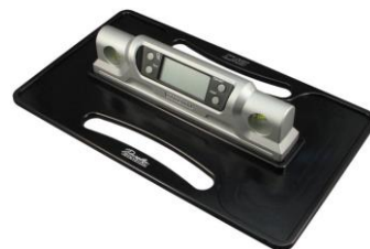
Figure 6: Official measuring device to check saddle inclination
