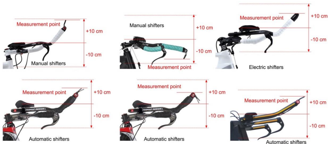
Figure 46: Points of measurement for the vertical limits of the fixed additional time trial extensions and any accessories
